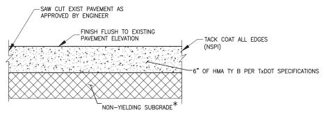
IF SOFT SPOTS ARE ENCOUNTERED AT A 6" DEPTH, THE CONTRACTOR SHALL TREAT THE EXISTING SUBGRADE WITH SACKS OF CEMENT, OR EXCAVATE FURTHER TO ACHIEVE A NON-YIELDING SUBGRADE. THIS SHALL BE CONSIDERED SUBSIDIARY TO THE PAVEMENT REPAIR PAY ITEM.
